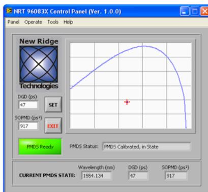
Main GUI for NRT-12033X: the cursor can be placed at any PMD state below the blue curve.
