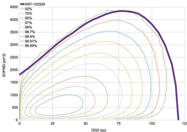
The NRT-12033X covers 99.99% of the states occurring in a 36 ps mean PMD fiber span. To the left, the joint probability density function of a 36 ps fiber is shown by the rainbow colored contours. The NRT-12033X can access all states below the dark blue curve, beyond the outmost contour. This wide DGD/SOPMD range, combined with the broad 33 GHz free spectral range enables the NRT-12033X to test, compare, design and deploy 10G/s and new generation 40G DP-QPSK transponders.
